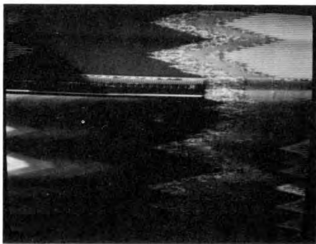
D2 MAC TV signal showing digital word synchronisation. Not resolvable on a 'normal' TV set.
